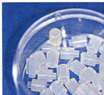
Fig. 2 Disposable caps cover the measuring probe to minimize the risk of cross contamination.
